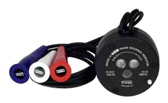
The K-7-1 Phase Sequence Indicator indicates the order of succession in time of the different voltage peaks of a multi-phase supply. The K-7-1 is used to make three-phase circuit installations or alterations as well as replacement installations of motors and generators. It can be used for making continuity tests of circuits of poly-phase systems. It is also valuable in making connections of power-factor meters, voltampere meters, watt and watthour meters and relays.
